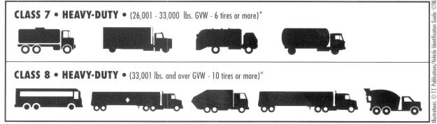
Classes 7 and 8 include a wide range of heavy vehicles, large delivery trucks, motor coaches, refuse trucks, cement mixers, all tractor trailer combinations including double trailers.
